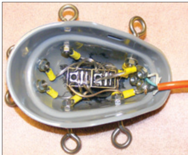
Figure 5 — Relay box assembled in a power entry PVC cover.
